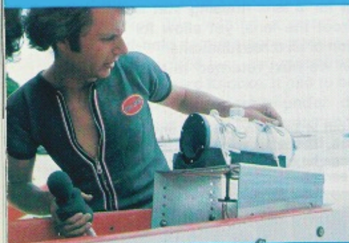
(LEFT) Joe Seamans checks installation of 50-foot-load gun camera in a waterproof housing mounted on bow of 16-foot canoe. (CENTER) As Tommy Holmes selects a good wave to ride in his canoe, he triggers the gun camera. The first time this sequence was tried, Holmes was flipped out of the canoe when a 20-foot wave broke over it. (RIGHT) Seamans uses the silent Arri to shoot boat-to-boat action.
